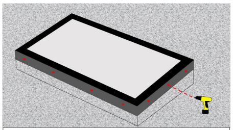
3) Pre drill fixing holes through aluminium and timber upstand/kerb at 100mm from each corner and then at regular intervals.
