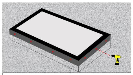
3) Pre drill fixing holes through aluminium and timber upstand/kerb at 100mm from each corner and then at regular intervals.
