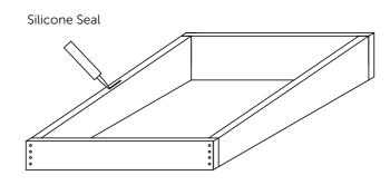
Lift the glazed rooflight onto the top of the kerb, keeping an equal spacing around the perimeter.
