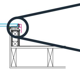
Fix the exterior trims around the perimeter of the rooflight using a rubber hammer if necessary.
